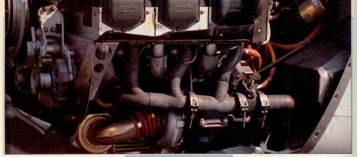
The cowl design gives up a few knots of speed to ensure adequate engine cooling, critical in a turbocharged airplane.
